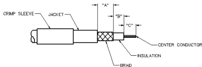
3. Assemble contact onto cable as shown.
