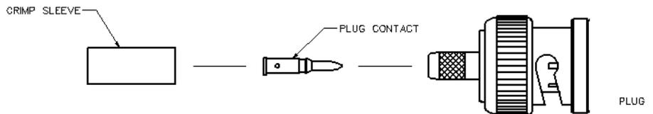
1. Identify connector parts. (3 piece parts)
